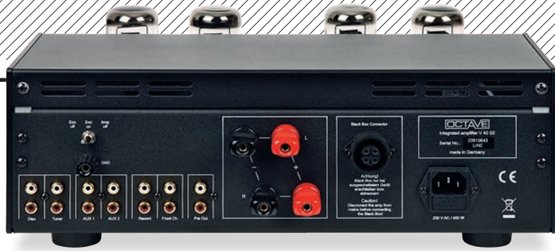
ABOVE: Three line ins are joined by tape, a line-level 'front ch' and pre outs. Fixed-tap speaker connections are via substantial 4mm posts. Note 'Black Box' connection
