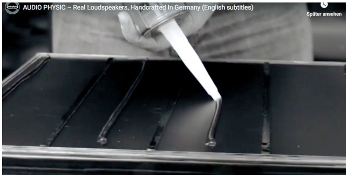
The permanently elastic acrylic is applied in Brilon by hand (Photo: Audio Physic)
