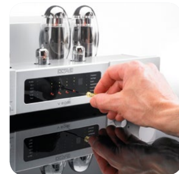
The LED indicator on the display simplifies adjusting the optimum bias current of the tubes.
