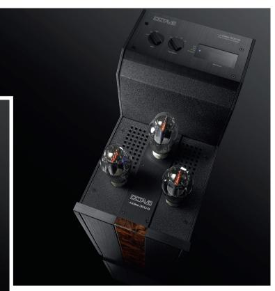
An energy management for the supply and heating voltages ensures a long valve life, a protection and overload system keeps safe from operating errors and valve malfunctions. The quiescent current of the three power valves is checked by a measuring device with a digital display.
